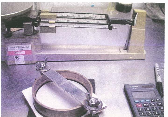
Water Absorption (Cobb Method)
